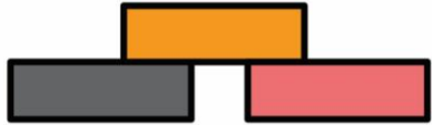
5. PLACING THE TOP UNIT ON BOTH GROUND FLOOR UNITS SUCH THAT IT GETS OPEN SPACE ON BOTH SIDES
