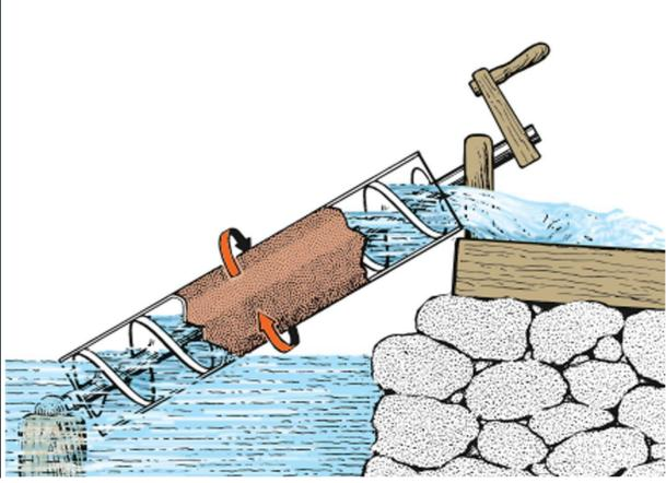
The Archimedes screw is one of the earliest hydraulic machines. A positive-displacement pump traps fluid from a source and then forces the fluid to move to a discharge location.
