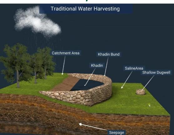
An ingenious construction designed to harvest surface runoff water for agriculture. Its main feature is a very long (100-300 m) earthen embankment built across the lower hill slopes lying below gravelly uplands.
