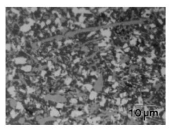
Fig. 1 Optical Micrograph of Al<sub>2</sub>O<sub>3</sub>–SiC<sub>w</sub>–TiC composite, where the bright grains are TiC particles, the *light-grey filaments* are the SiC whiskers, and the *dark-grey background* is the alumina matrix [4]
