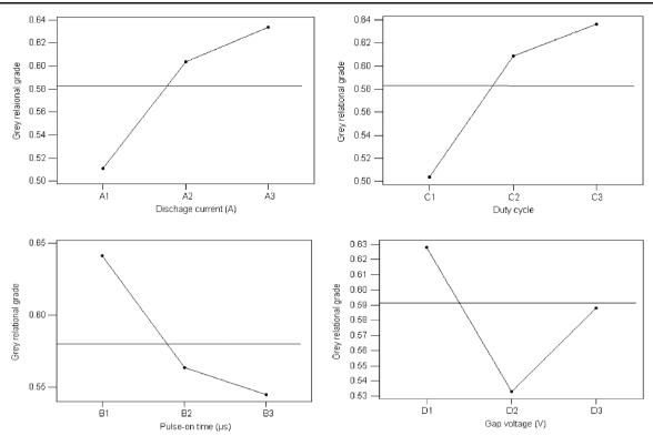
Fig. 3 Effect of EDM parameters on the multi-performance characteristics
