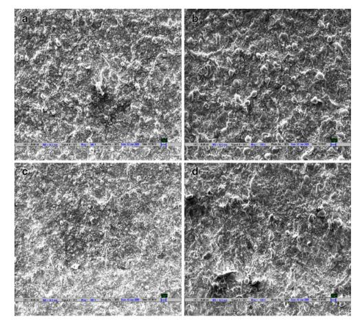
Fig. 5 EDMed surface characteristics of  $Al_2O_3$ -SiC<sub>w</sub>-TiC ceramic composite at a duty cycle of 0.64 and a gap voltage 70 V: **a** 3 A, 50  $\mu$ s, **b** 3 A, 150  $\mu$ s, **c** 7 A, 50  $\mu$ s, **d** 7 A, 150  $\mu$ s
