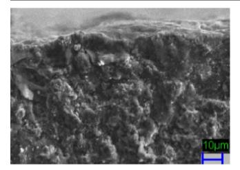
Fig. 6 SEM micrographs shows the formation of the recast layer
