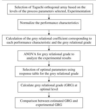
Fig. 2 Grey relational analysis to optimise the process with multipleperformance characteristics
