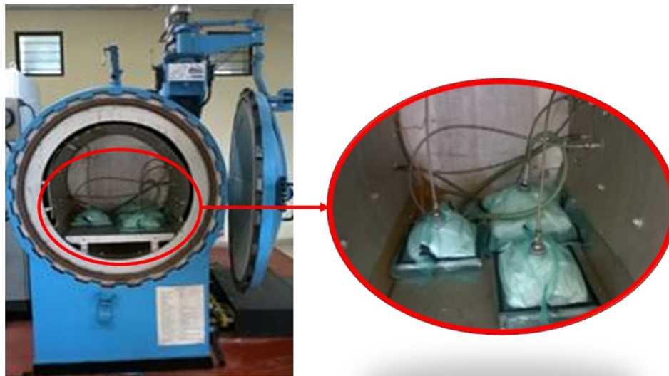
Fig. 2. Parabolic antenna reflectors cured in an autoclave machine.
