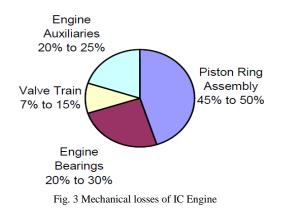
Our main focus is to reduce the losses due to piston rings friction to decrease the emissions of engine.
