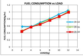
Fig. 8 Fuel Consumption Vs Load
