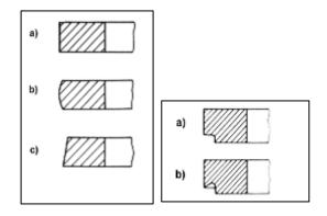
Fig. 4 & Fig. 5 Compression ring cross-section (ISO 6621-1).
