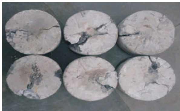
Figure 8. Impact Strength of FRAAC Specimen
