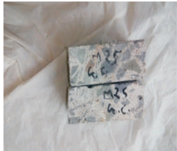
Figure 9. FRAAC Specimen after Abrasion Test
