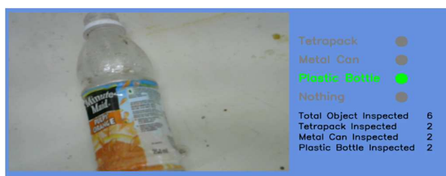
Fig. 9. Result image correctly identifies plastic bottle
