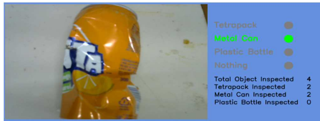
Fig. 8. Result image correctly identifies metal can
