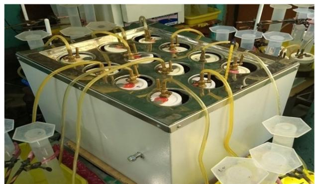
**Fig. 1** Experimental set-up for anaerobic co-digestion FVW and AS
