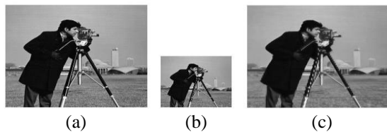
Figure 10. (a) HR image (b) LR Image (c) Reconstructed Image by SCDL with \lambda=0.0024553 by GCV
