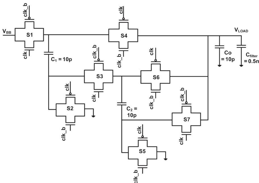
Fig. 10. Circuit diagram of 3:1 switched capacitor converter.
