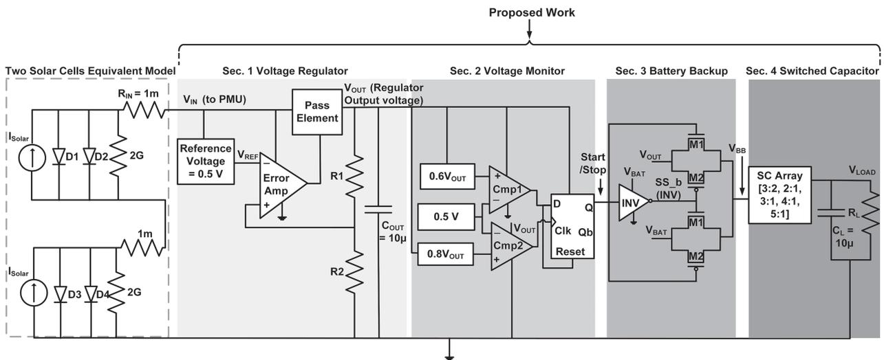
Fig. 2. Circuit diagram of the proposed work.
