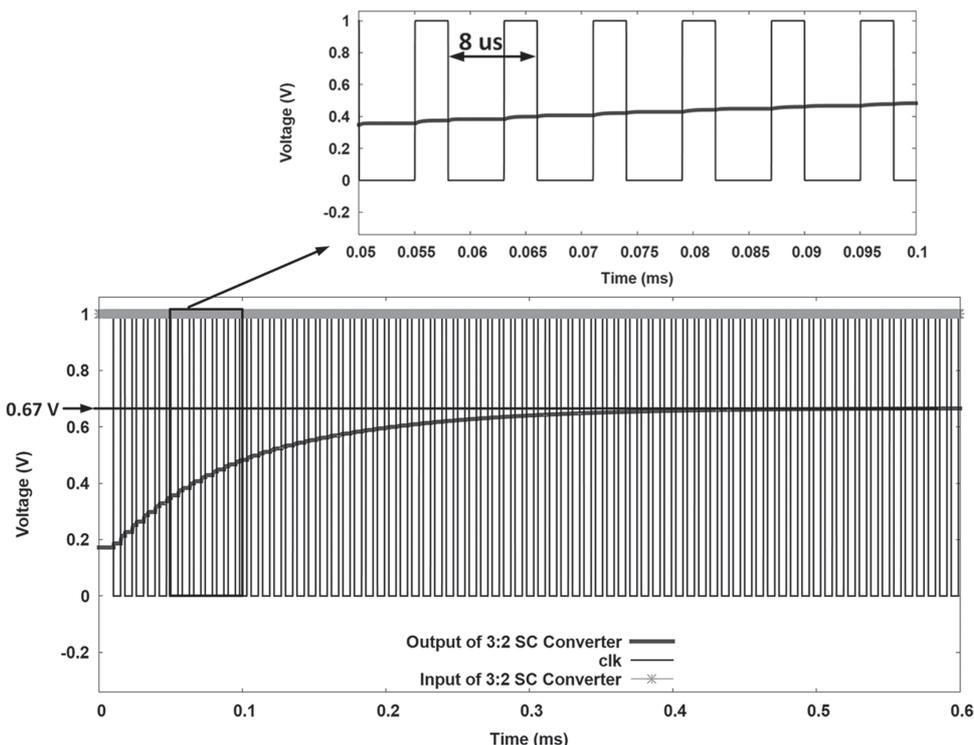
Fig. 6. Transient response of 3:2 switched capacitor converter.
