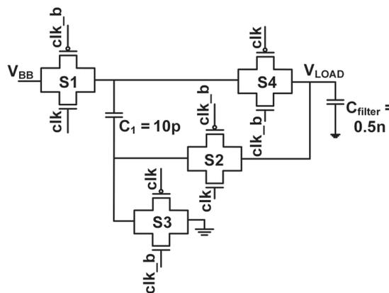
Fig. 7. Circuit diagram of 2:1 switched capacitor converter.
