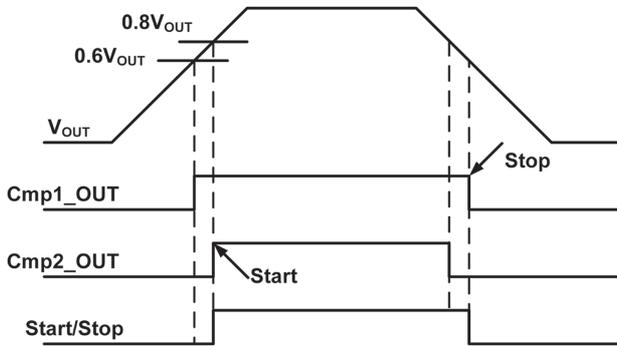
Fig. 4. Ideal response of the voltage monitor.
