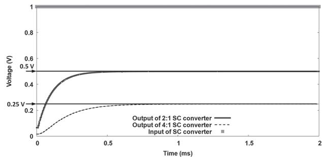
Fig. 9. Transient response of 2:1 and 4:1 switched capacitor converters.
