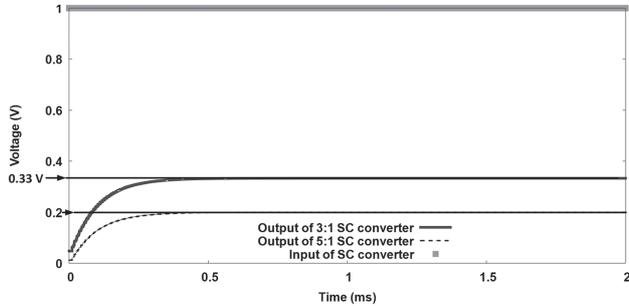
Fig. 13. Transient response of 3:1 and 5:1 switched capacitor converters.
