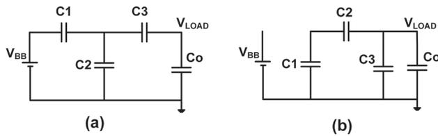
Fig. 12. Equivalent circuit for (a) phase 1 (b) phase 2 of 5:1 switched capacitor converter.
