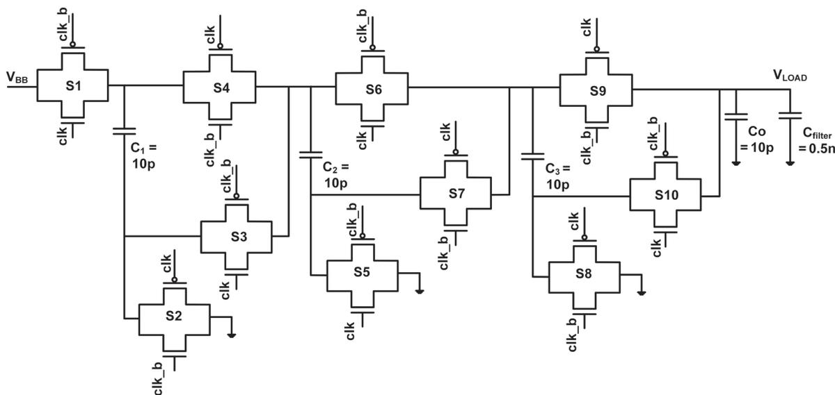
Fig. 11. Circuit diagram of 5:1 switched capacitor converter.
