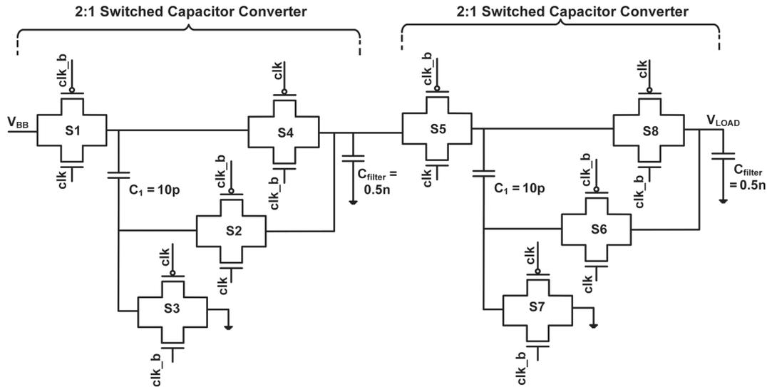
Fig. 8. Circuit diagram of 4:1 switched capacitor converter.
