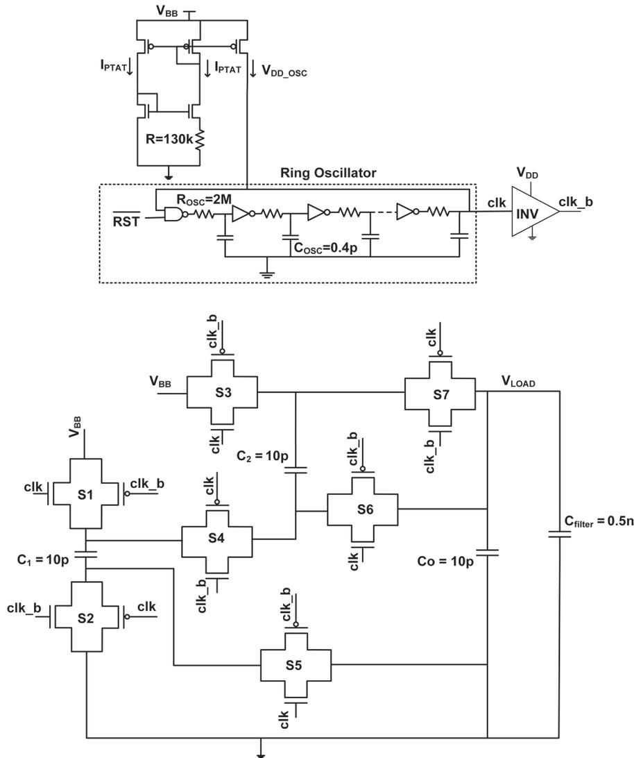
Fig. 5. Circuit diagram of 3:2 switched capacitor converter.
