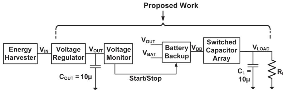
Fig. 1. Block diagram of the proposed PMU.
