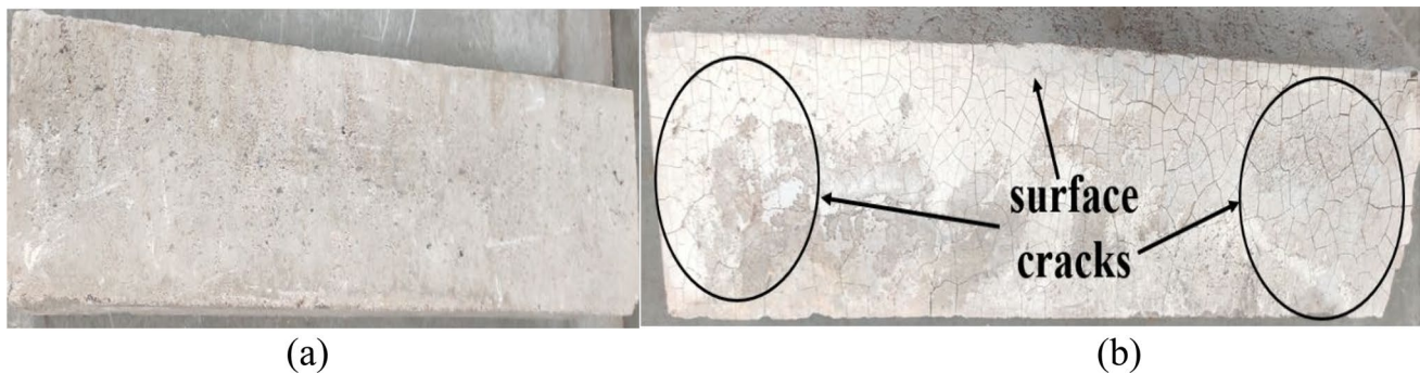
Fig. 10 Control concrete a at room temperature b at an exposure of 800 °C
