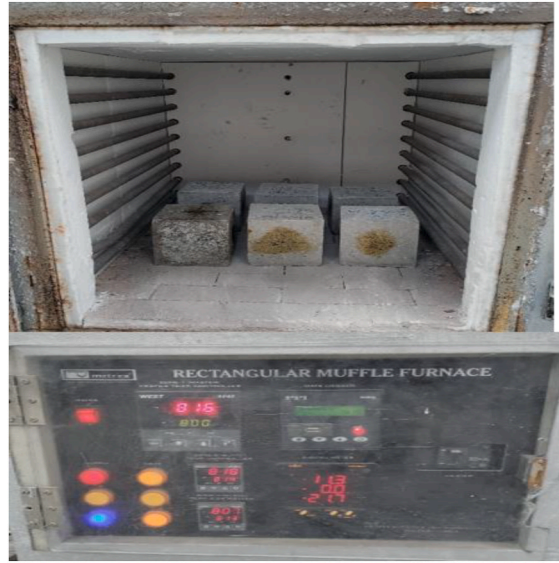
Fig. 4. Muffle furnace used in the study.
