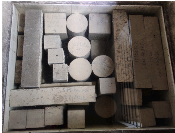
Fig. 6. Curing of RAC specimens in curing chamber.
