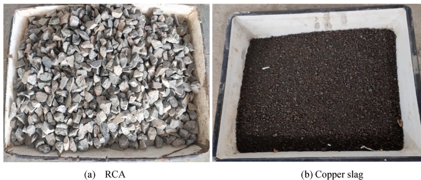
Fig. 2. Waste materials used in the research work.
