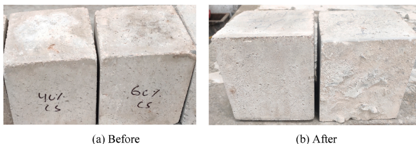
Fig. 15. Specimens exposed to sulphate attack.
