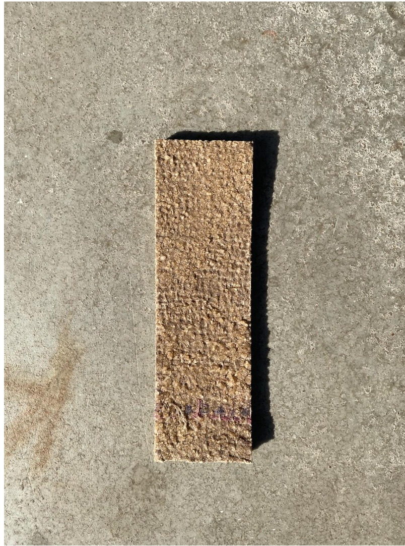
Testing the sample we created that is 7 layered took load of 700+ kgs.
