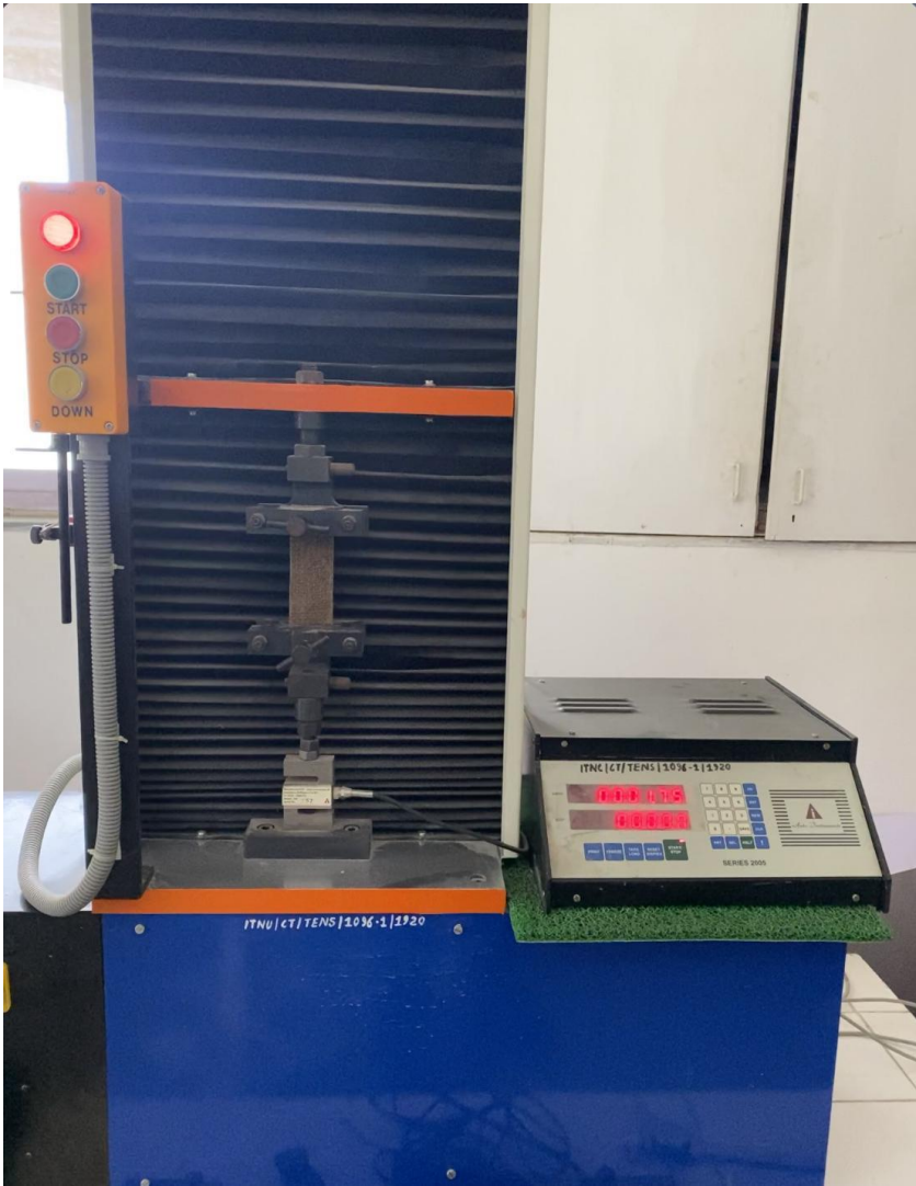
Testing the sample we created that is 7 layered took load of 700+ kgs.
