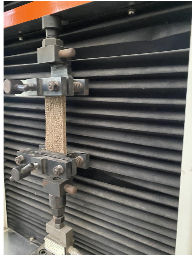
Testing the sample we created that is 7 layered took load of 700+ kgs.
