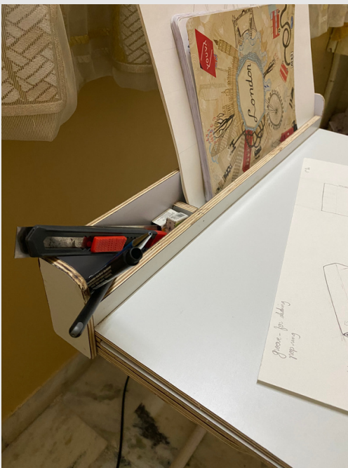
An Organizer on the top base where the basic stationery and sheets and book of Size A3 can kept, which will be easily accessible .
