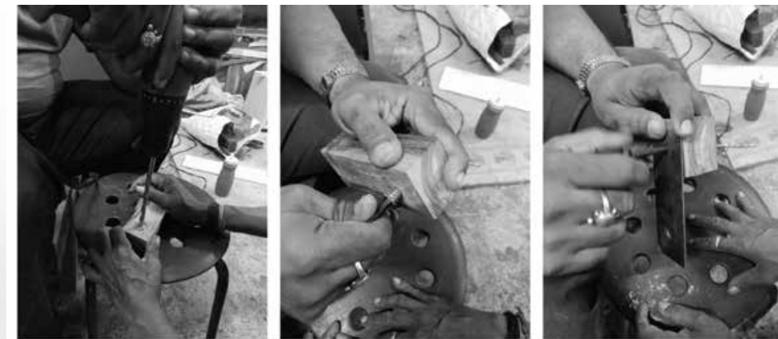
CSK allen bolt and flanged hex drive nut used to fix metal plates to wood.
