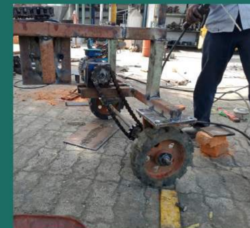
Stage 2 - • Attaching the motors and the compressor. • Changing the wheels , because the prior once were not able to take the load . Poor grip and less durable • Added Tubeless tyres
