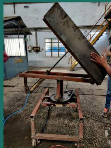
Stage 1 :- Attaching hydraulic cylinder and testing it . We could run the cart manually.
