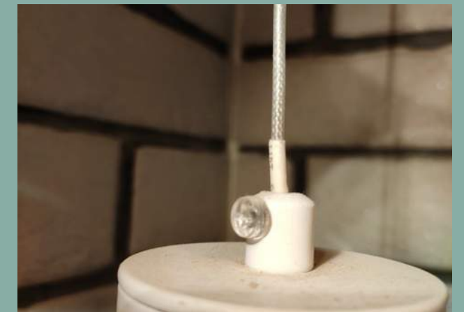
Joint at the lid using the nylon wire suspensions
